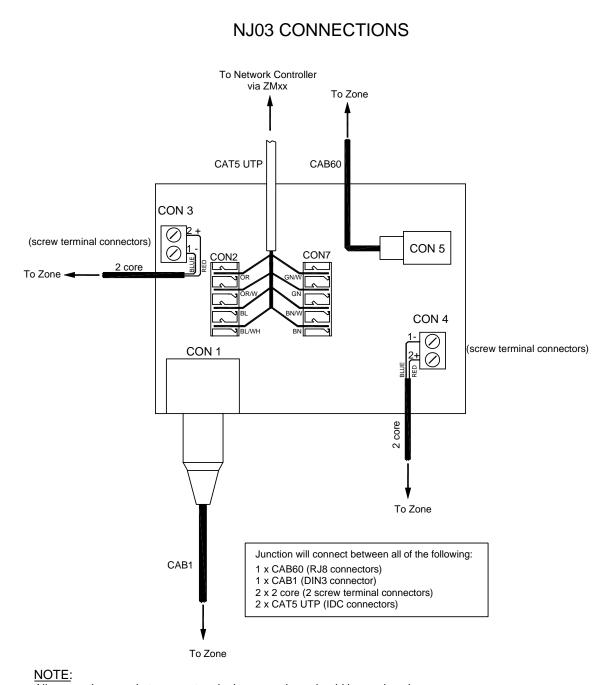
All connections made to screw terminals connections should be made using unscreened 2 core cable. (eg 7/0.2-2)
