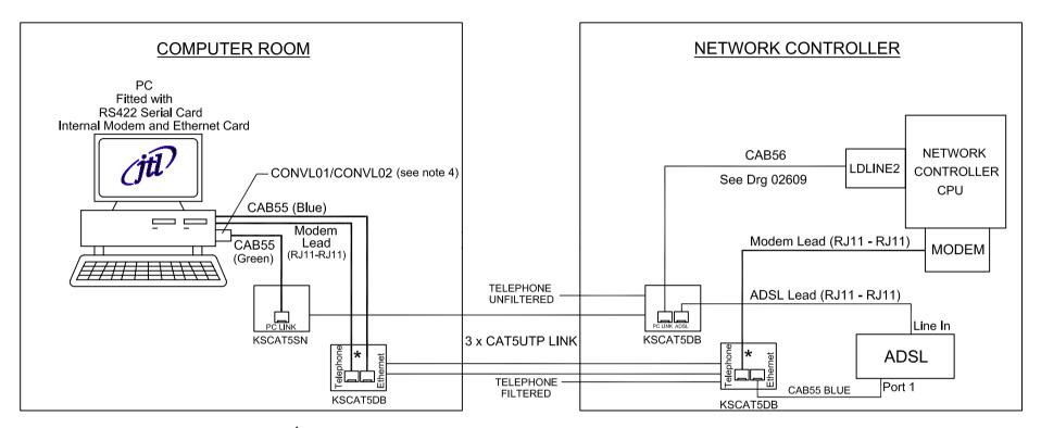
\*RJ11 Plug fits into the centre of an RJ45 Socket without need for BT adapter.
