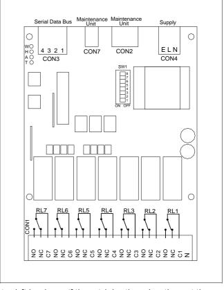
If the watchdog timer does time out then the indicator will be extinguished and the card reverts to standby mode. In standby mode all outputs can be directly operated by bitswitches (SW1) mounted on the interface card.
