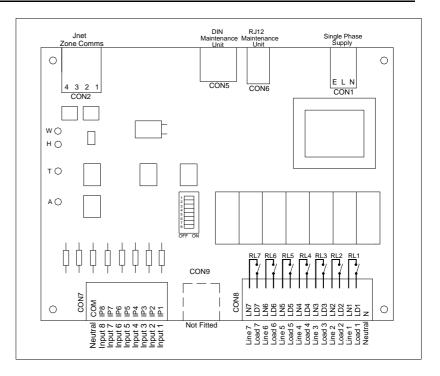
Four LEDs are located in the top left hand corner of the PCB. These are for diagnostic purposes.
